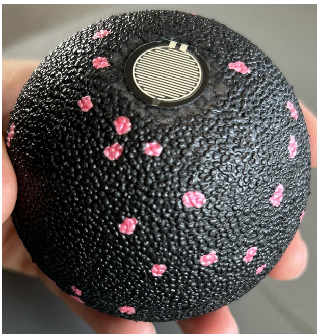
Figure 2. Current prototype of the Sound Ball.
